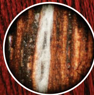
Fig 3: Hybrid System (Conversion Varnish under Waterborne)
