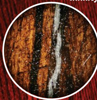
Fig 3: Hybrid System (Conversion Varnish under Waterborne)
